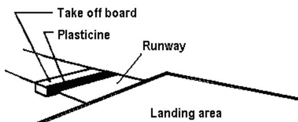
**THE LANDING AREA:** This should be at least 2.75m wide and the distance from the take-off line to the end of the landing area should be at least 10m. The surface of the sand in the landing area should be level with the top of the take-off board.
